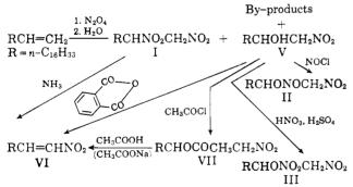
Addition of dinitrogen tetroxide to 1-octadecene, 10 hydrolysis, and subsequent fractional crystallization gave pure 1-nitro-2-octadecanol, 10 V, and 1,2-dinitrooctadecane, I, of > 90% purity; infrared spectra and elemental analyses of I proved the complete absence of V and 1-nitro-2-octadecyl nitrate, III, and the presence of less than 10% 1-nitro-1-octadecene, VI; the latter
